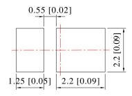
Unit: mm Tolerance: ±0.10mm
