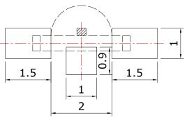
Unit: mm Tolerance: ± 0.10mm
