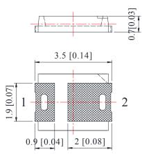
**Recommended Soldering Pad Dimensions**
