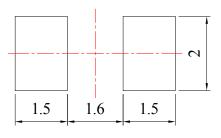
Unit: mm Tolerance:  $\pm 0.10$ mm
