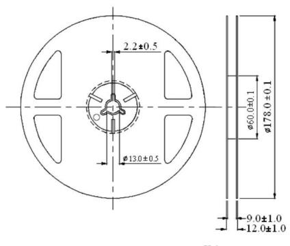
Unit: mm Tolerance:  $\pm 0.25$ mm
