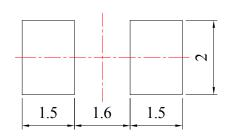
Unit: mm Tolerance: ± 0.10mm
