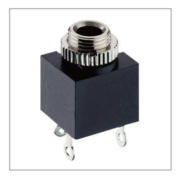
Jack chassis socket acc. to JIS C 6560 JC35J2B, 3.5 mm, 2 poles/mono, with break contact and solder eyes, also for printed circuit boards, for back side mounting
