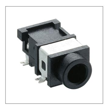
Jack chassis socket acc. to JIS C 6560 JC35J3A, 3.5 mm, 3 poles/stereo, angular version, for printed circuit boards, surface mounting technology (SMT)
