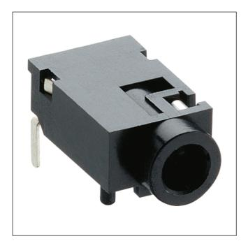
Jack chassis socket acc. to JIS C 6560 JC35J2B, 3.5 mm, 2 poles/mono, angular version, with break contact, for printed circuit boards
