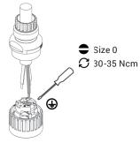
Unscrew the PE-contact, insert the PE-conductor and tighten again.
