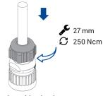
Screw the cable gland to the connector body.
