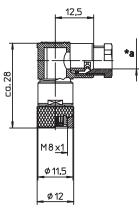
\*a O-Ring \*b Screw joint for cable
