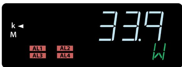
Automatically displayed unit of measured value and symbol of multiplier kilo, mega.
