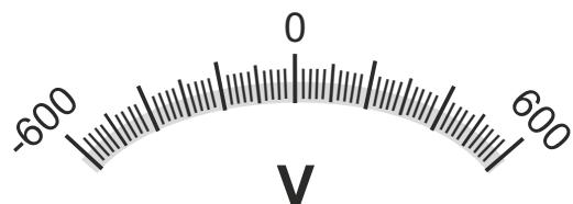
Bidirectional voltage measurement in a wide range of  $\pm 600\text{V}$  (maximum indication range  $\pm 1200\text{V}$ ) and bi-directional current measurement through a shunt. This function is useful, among others when monitoring the parameters of an energy storage system.
