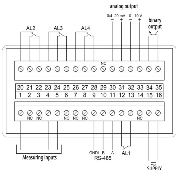
Description of signals on the connector strips
