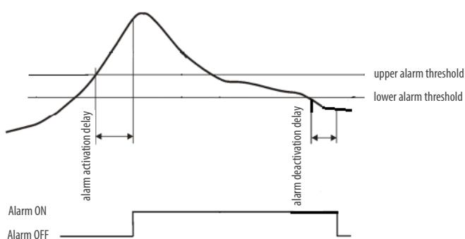
$t \geq$  time delay --> Alarm activated
