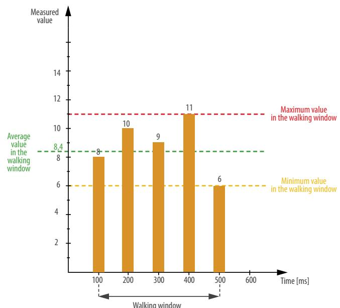
Programmed averaging time according to the walking window algorithm with a given averaging time. This function is useful for measuring signals with high dynamics.
