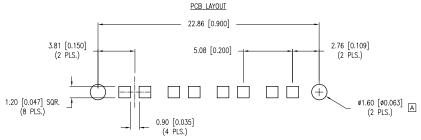
\*UNLESS OTHERWISE SPECIFIED TOLERANCES PER DECIMAL PRECISION ARE: X=±1 (±0.039), X.X=±0.5 (±0.020), X.XX=±0.25 (±0.010), X.XXX=±0.127 (±0.005). LEAD SIZE=±0.05 (±0.002), LEAD LENGTH=±0.75 (±0.030). MIN= +DECIMAL PRECISION WAX.= +0.00 -DECIMAL PRECISION UNCONTROLLED DOCUMENT
