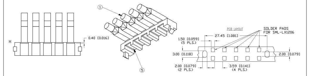
\*UNLESS OTHERWISE SPECIFIED TOLERANCES PER DECIMAL PRECISION ARE: X=±1 (±0.039), X.X=±0.5 (±0.020), X.XX=±0.25 (±0.010), X.XXX=±0.127 (±0.005). LEAD SIZE=±0.05 (±0.002), LEAD LENGTH=±0.75 (±0.030). MIN= +DECIMAL PRECISION MAX.= +DECIMAL PRECISION LINCONTROLLED DOCLIMENT
