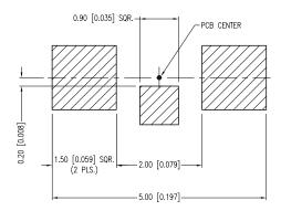
\*UNLESS OTHERWISE SPECIFIED TOLERANCES PER DECIMAL PRECISION ARE: X=±1 (±0.039), X.X=±0.5 (±0.020), X.XX=±0.25 (±0.010), X.XXX=±0.127 (±0.005). LEAD SIZE=±0.05 (±0.002), LEAD LENGTH=±0.75 (±0.030). MIN=  $\frac{+0.001}{-0.000}$  MAX.=  $\frac{+0.001}{-0.000}$  MA UNCONTROLLED DOCUMENT
