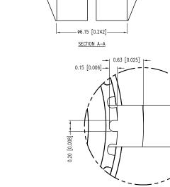
\*UNLESS OTHERWISE SPECIFIED TOLERANCES PER DECIMAL PRECISION ARE:  $x=\pm1$  (±0.039),  $x.x=\pm0.5$  (±0.020),  $x.xx=\pm0.25$  (±0.010),  $x.xxx=\pm0.127$  (±0.005). LEAD SIZE=±0.05 (±0.002), LEAD LENGTH=±0.75 (±0.030). MIN=  $\frac{+0.00}{-0.00}$  MAX.=  $\frac{+0.00}{$
