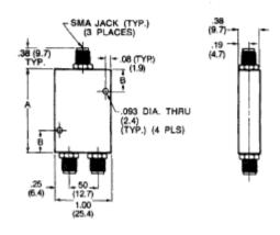
Note: All dimensions are  $\pm\,$  .020, except mounting hole diameters (±  $\,$  .005) and mounting hole location (±  $\,$  .010) .
