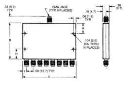
All dimensions are  $\pm$  .020, except mounting hole diameters ( $\pm$ .005) and mounting hole location ( $\pm$  .010).
