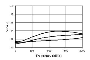
VSWR vs. Frequency Reference Loss, 0.5, 1, 2 dB Bits
