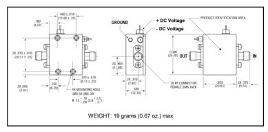
\* Dimensions are inches (millimeters) ±0.015 (0.38) unless otherwise specified.
