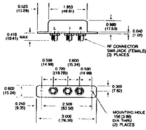
DIMENSIONS ARE IN INCHES (MILLIMETERS) ± 015 ( 38) UNLESS OTHERWISE SPECIFIED
