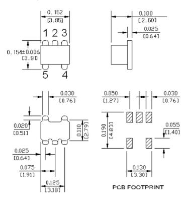
Dimensions are inches (millimeters)  $\pm 0.015$  (0.38) unless otherwise specified. Drawing not to scale.
