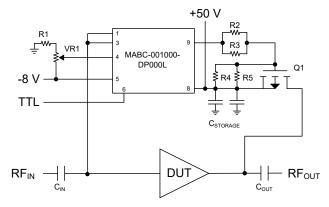
Figure 1. Fixed Gate/Pulsed Drain Biasing
