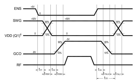
6. Q1 refers to an external p-Channel HEXFET that pulses the drain of the DUT. See Applications Section for more information.
