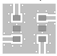
10.Recommended PCB layout shown above uses 1.6 mm FR4, rounded coplanar wave guide, transmission line width 0.70 mm and gap 0.57 mm.
