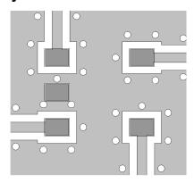
Recommended PCB layout shown above uses 1.6 mm FR4, Grounded coplanar wave guide, transmission line width 0.70 mm and gap 0.57 mm.
