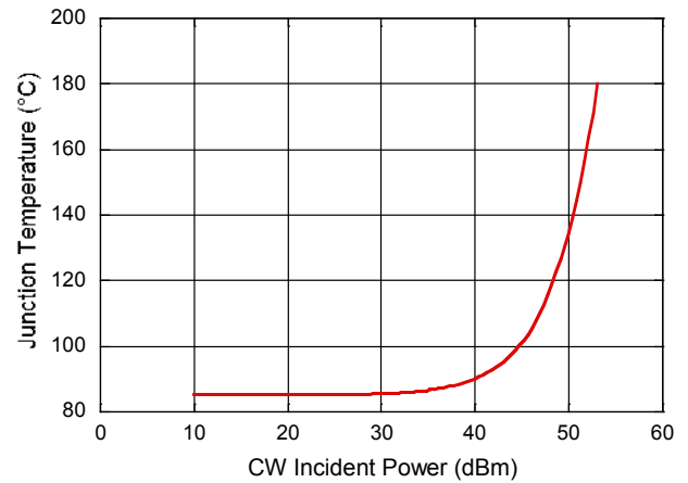
Junction Temperature 1 GHz, CW @ T_A = +85^\circ\text{C}
