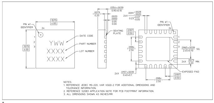
Reference Application Note S2083 for lead-free solder reflow recommendations. Meets JEDEC moisture sensitivity level 1 requirements. Plating is 100% matte tin over copper.
