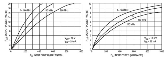
Figure 2. Output Power versus Input Power
