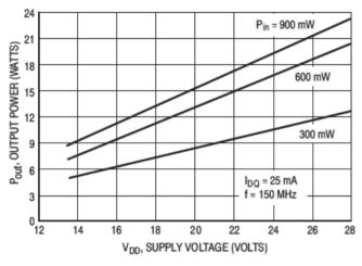
Figure 6. Output Power versus Supply Voltage
