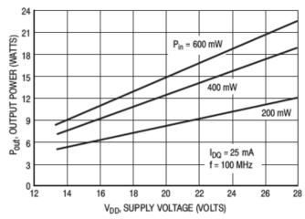
Figure 4. Output Power versus Input Power
