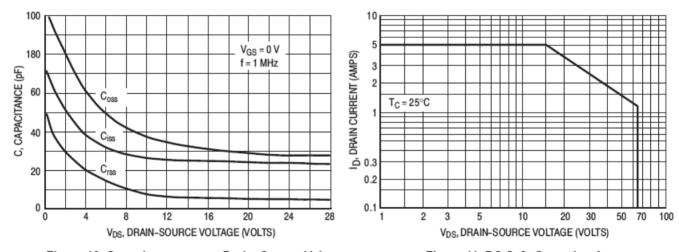
Figure 10. Capacitance versus Drain-Source Voltage
