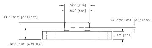
Unless otherwise noted, tolerances are inches  $\pm .005$ " [millimeters  $\pm 0.13$ mm]
