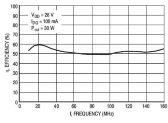
Figure 14. Drain Efficiency versus Frequency
