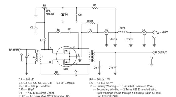
Figure 1. 30-150 MHz Test Circuit
