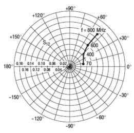
Figure 20.  $S_{12}$ , Reverse Transmission Coefficient versus Frequency  $V_{DS} = 28 \text{ V}$   $I_D = 0.5 \text{ A}$
