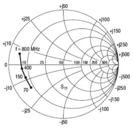
Figure 19. S<sub>11</sub>, Input Reflection Coefficient versus Frequency  $V_{DS} = 28 \text{ V}$  I<sub>D</sub> = 0.5 A
