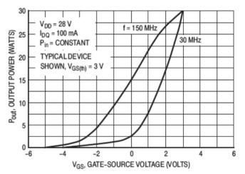
Figure 15. Output Power versus Gate Voltage
