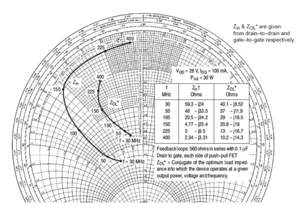
Figure 18. Input and Output Impedance
