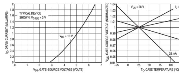
Figure 8. Drain Current versus Gate Voltage (Transfer Characteristics)\*
