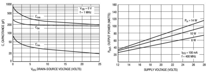
Figure 7. Capacitance versus Drain-Source Voltage
