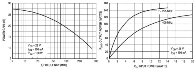
Figure 10. Power Gain versus Frequency
