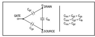
The Ciss givenin the electrical characteristics table was measured using method 2 above. It should be noted that-Ciss, Coss, Crss are measured at zero drain current and are provided for general information about the device. They are not RF design parameters and no attempt should be made to use them as such.
