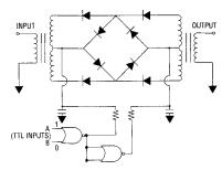
DC volts:  $5 \pm 1\%$  nominal; DC current 45 mA TTL logic inputs "0" = 0 volt "1" = 5 volts nominal 2 volts minimum 6 volts maximum
