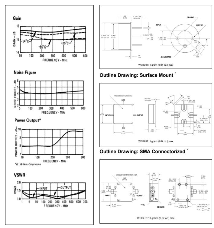
\* Dimensions are inches (millimeters) ±0.015 (0.38) unless otherwise specified.
