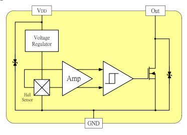
Note: Static sensitive device; please observe ESD precautions. Reverse  $V_{DD}$  protection is not included. For reverse voltage protection, a 100  $\Omega$  resistor in series with  $V_{DD}$  is recommended.
