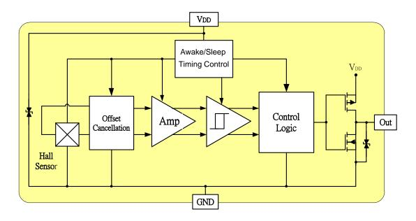
*Note*: Static sensitive device; please observe ESD precautions. Reverse  $V_{DD}$  protection is not included. For reverse voltage protection, a 100  $\Omega$  resistor in series with  $V_{DD}$  is recommended. MH254, HBM > ±4KV which is verified by third party lab.
