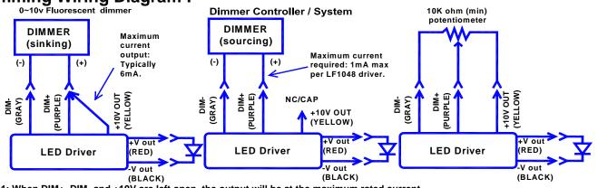
Note1: When DIM+, DIM- and +10V are left open, the output will be at the maximum rated current. Note2: When input is greater than 18VDC, the Vf (forward voltage) has to be at least 2VDC higher than the input voltage. Note3: LD1060-100-C0600 does comply to UL8750 safety standard but not certified at the moment.
