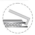
1. Hook Talon clip under one side of the BGA chip set.
