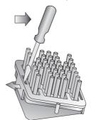
3. Carefully disengage opposite side clip and remove the heat sink assembly from the chip set.
