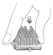
4. Press firmly down to make sure Talon clips fully engage edges of chip set. Installed heat sink assembly should not move around easily...
