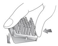
2. Rotate assembly down until opposite side clip engages edge of BGA chip set.
