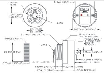
NDTE A: TERMINALS-032 BRASS TIN PLATED, TAPPED FOR #6-32 SCREW. TWO #6-32 NICKEL PLATED BRASS SCREWS INCLUDED. WILL ACCEPT 1/4\* DUICK CONNECT. NOTE B: MOUNTING- REMOVE BLACK PLASTIC NUT AND INSERT THREADED FRONT THROUGH LES' HOLE PUNCHED IN PANEL, IF DRIENTATION IS NEDED, NOTE LOCKING FLATS ON DRAWING. SCREW NUT BACK ON. DO NOT OVERTIGHTEN.
