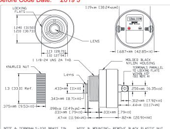
IDTE A: TERMINALS-032 BRASS TIN PLATED, TAPPED FIR #6-32 SCREW. TWD #6-32 NICKEL PLATED BRASS SCREWS INCLUDED. WILL ACCEPT 1/4\* QUICK CONNECT.
