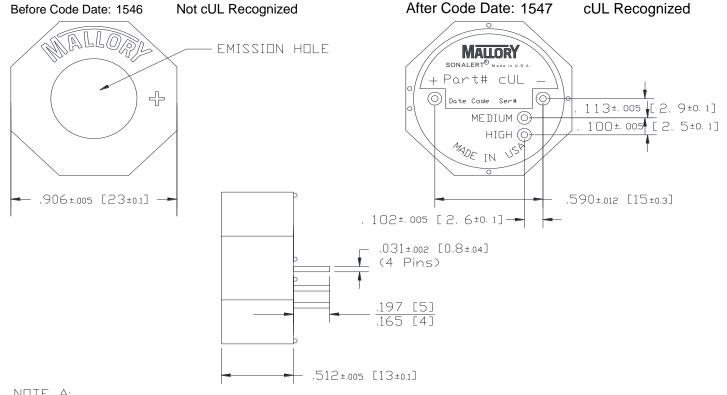
NOTE A: TERMINALS - .031" DIA. NICKEL/TIN COATED BRASS. NOTE B:
