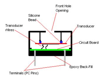
The above cross section picture shows the basic elements used in a piezoelectric audible alarm. The area in front of the transducer element including the front hole opening forms an acoustic cavity that lets the sound radiate out with the most efficiency (i.e. loudest sound level). If the alarm is an indicator that contains a circuit board, the circuit board is attached to the piezoelectric sounder element via soldered wires.
