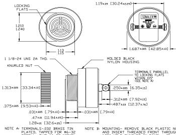
NOTE A: TERMINALS-032 BRASS TIN PLATED, TAPPED FOR #6-32 SCREW. TWD #6-32 NICKEL PLATED BRASS SCREWS INCLUDED, WILL ACCEPT 1/4\* QUICK CONNECT. NOTE B: MOUNTING- REMOVE BLACK PLASTIC NUT AND INSERT THREADED FRONT THROUGH 1.25' HOLE PUNCHED IN PANEL, IF DRIENTATION IS NEEDED, NOTE LOCKING FLATS ON DRAWING. SCREW NUT BACK ON. DO NOT OVERTIGHTEN.
