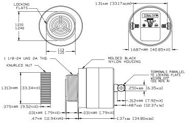
NOTE A: TERMINALS-.032 BRASS TIN PLATED, TAPPED FOR #6-32 SCREW. TWO #6-32 NICKEL PLATED BRASS SCREWS INCLUDED. VILL ACCEPT 1/4\* QUICK CONNECT. NOTE B: MOUNTING- REMOVE BLACK PLASTIC NUT AND INSERT THREADED FRONT THROUGH 1.25' HOLE PUNCHED IN PANEL, IF DRIENTATION IS NEEDED, NOTE LOCKING FLATS ON DRAWING. SCREW NUT BACK ON. DO NOT OVERTIGHTEN.
