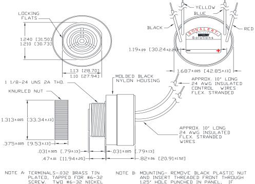
NDTE A: TERMINALS-.032 BRASS TIN PLATED, TAPPED FOR #6-32 SCREW. TWO #6-32 NICKEL PLATED BRASS SCREWS INCLUDED. WILL ACCEPT 1/4" QUICK CONNECT.
