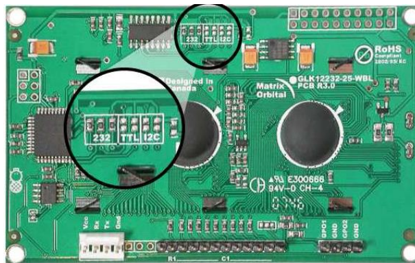
Figure 12: Protocol select Jumpers
