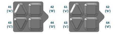
Figure 10: Default Tactile Key Down Values Figure 11: Default Tactile Key Up Values
