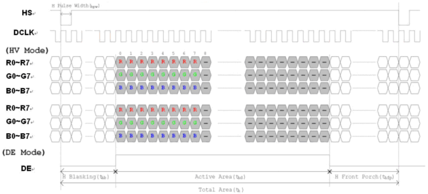
Figure 5: Horizontal Input Timing Diagram
