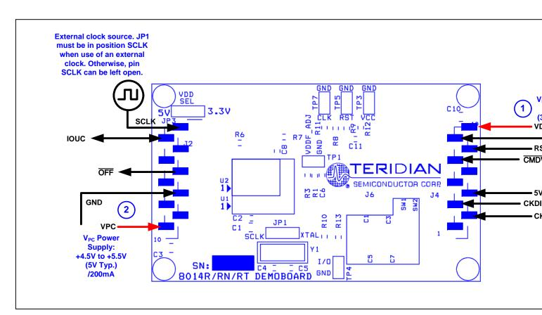
Figure 2: 73S8014R/RN/RT Demo Board: Basic Connections
