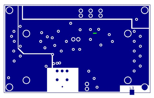
Figure 9: TERIDIAN 73S8014R/RN/RT 20SO Demo Board: Middle Layer 2, Supply Plane.
