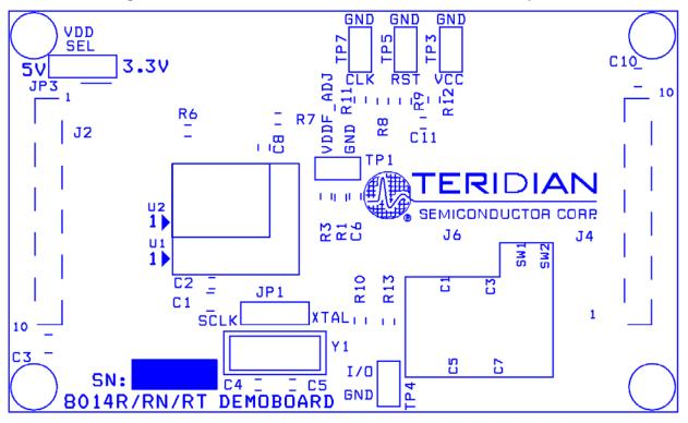
Figure 5: TERIDIAN 73S8014R/RN/RT 20SO Demo Board: Top View
