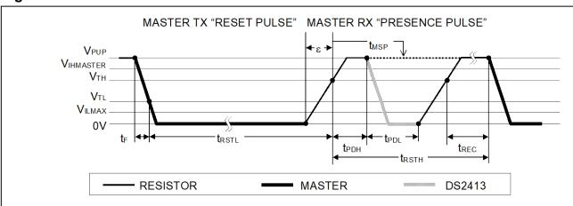
Figure 11. Initialization Procedure: Reset and Presence Pulse
