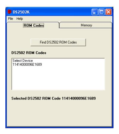
The ROM Codes Tab displays the ROM Codes of all the DS2502s that are found on the 1-Wire bus. The user can refresh the list of ROM Codes by left-clicking on the Find DS2502 ROM Codes button. This will initiate a Search ROM sequence to find all of the 1-Wire devices with the family code of the DS2502.
