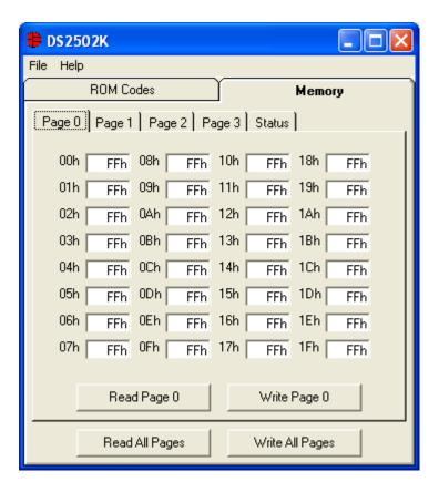
The Memory Tab gives the user access to read the contents of all of the Memory inside the DS2502. Left-clicking the Write Page X or Read Page X buttons will access the device for the specific page that is displayed. Left-clicking on the Read All Pages or Write All Pages will access Pages 0-3 and the Status registers.
