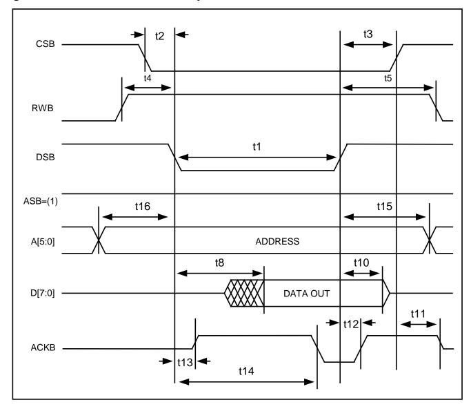
Figure 9-6. Motorola Mux Read Cycle
