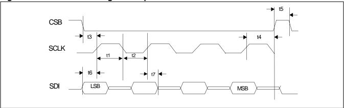
Figure 9-10. Serial Bus Timing Read Operation with CLKE = 0
