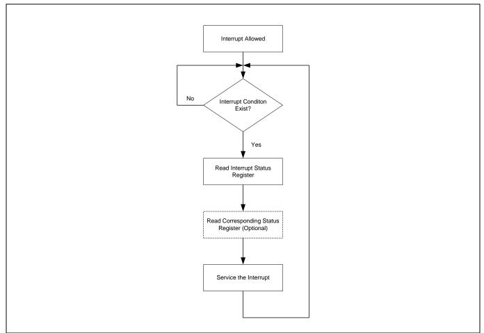
Figure 5-4. Interrupt Handling Flow Diagram
