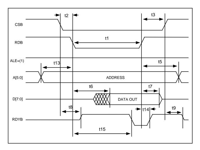
Figure 9-2. Intel Mux Read Cycle
