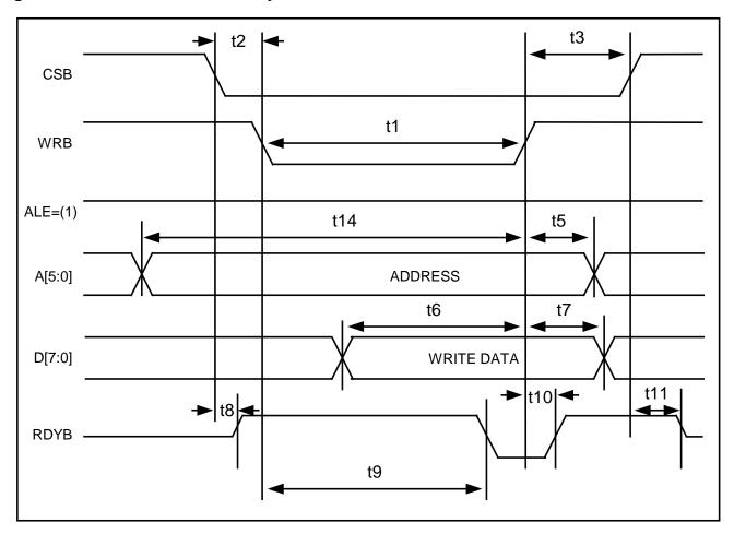
Figure 9-4. Intel Mux Write Cycle
