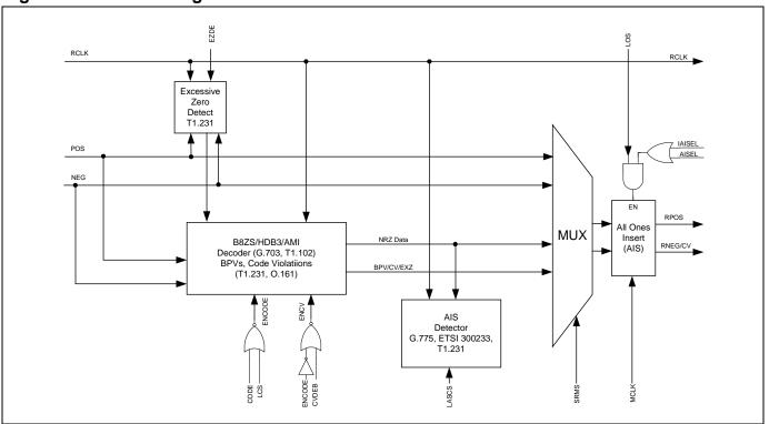
Figure 3-3. Transmit Logic Detail
