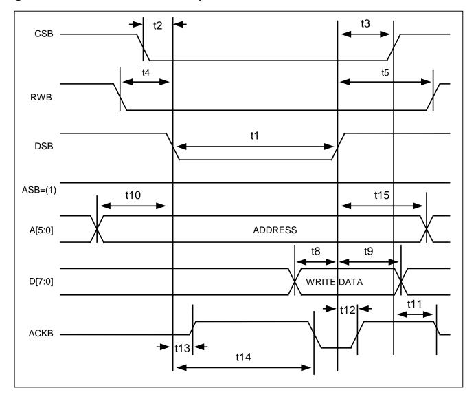
Figure 9-8. Motorola Mux Write Cycle
