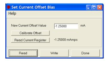
The Current Offset Bias can be entered into the text box and then written to the device by left-clicking on the Write button. A message box will be displayed asking if new offset should be copied to EEPROM. If Yes is clicked, a 15V programming voltage will need to be connected to the VPROG pin, as described in the Memory section below.
