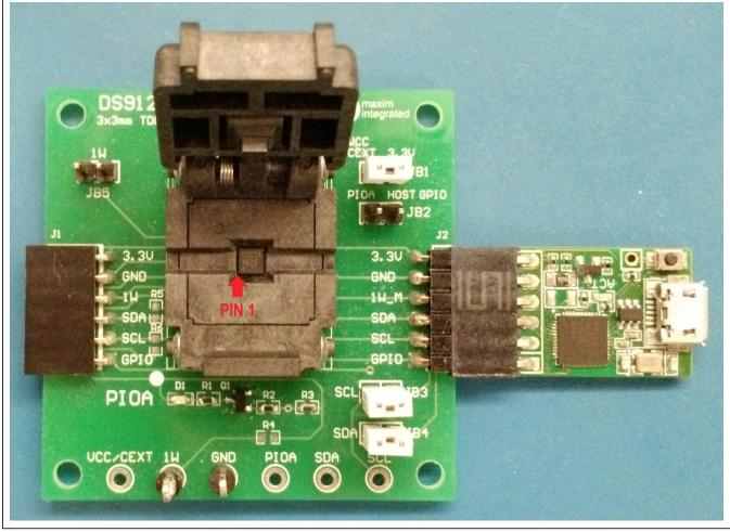
Figure 1. Orientation in Burn-In Socket
