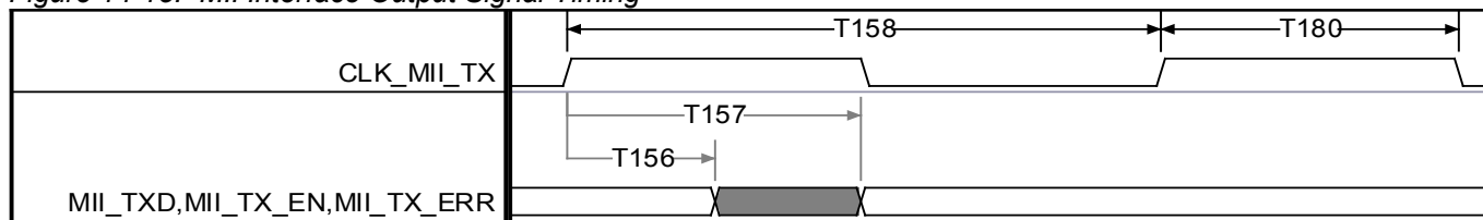
Figure 14-15. MII Interface Output Signal Timing
