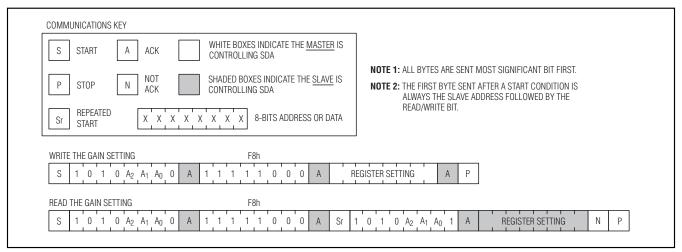
Figure 4. I<sup>2</sup>C Communication Examples
