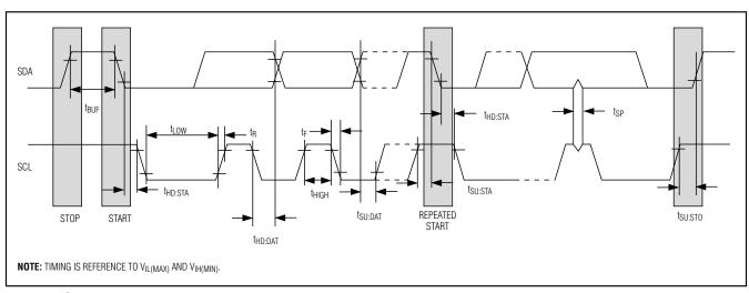
Figure 3. I<sup>2</sup>C Timing Diagram
