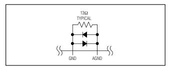
Figure 5. Internal Ground Connections
