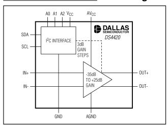
low-current (ISTBY) consumption state. Unlike mute mode, however, standby mode is intended for use when no input signal is present. While in standby mode, the DS4420 maintains input and output common-mode bias voltages. The device produces no audible clicks or pops when entering or exiting the standby state. The time required for the output to become active when exiting standby mode is specified as tpu.
