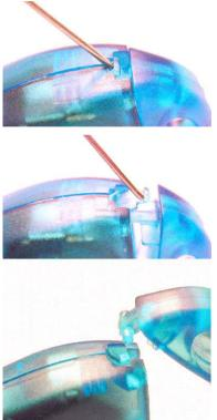
\*Note: The data contact faces down and away from the embossed 'i'. Once the <u>iButton</u> is inserted in the enclosure, snap the end cap over it. The end cap is removed by depressing the release tab with a paper clip, swinging it fully open, and sliding out the hinge.
